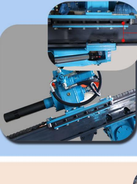
The newly designed rotary head, hydra ulic four-speed 0-110rpm,low-speed hi gh-torque, high-speed low-torque, adap t to various working conditions, and the rotary spindle will never wear. Lengthened wear-resistant plate and h
